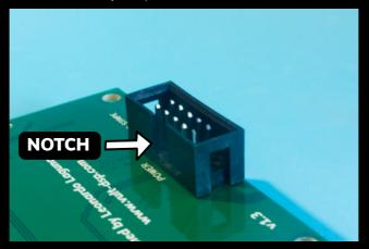
Use the same procedure as for the headers: solder one pin, verify that the connector is correctly placed and then solder the remaining pins.
