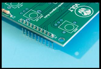
**IMPORTANT**: verify that the pins are correctly placed and that the angle is 90 degrees otherwise it will not be possible to connect the main board.
