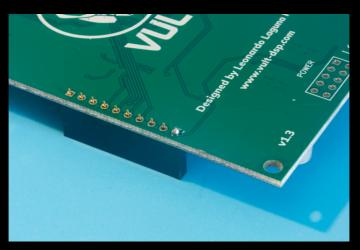
Verify that the header is correctly placed before soldering the rest. The header should stand at 90 degrees.
