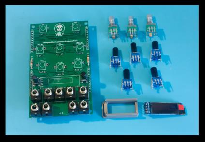
As preparation, remove the nuts from the potentiometers if they are placed.
