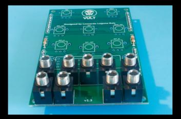
Gently tight two nuts on the jacks that are soldered. With all the jacks in place, turn the board around and solder all of them.
