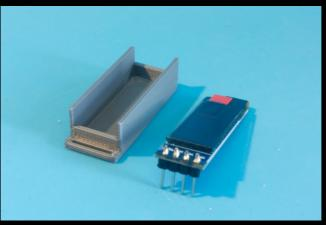
The holder has a small slot where the pins of the screen go. Carefully insert the screen and push it to the bottom until it sits correctly in the holder.
