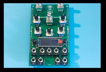
Once you solder the pins of the screen, carefully clean the flux residuals of that section.
