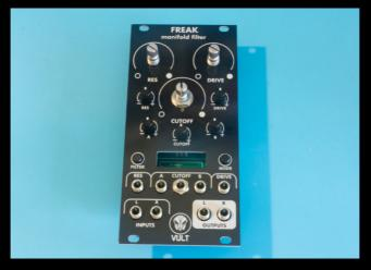
**IMPORTANT**: verify that all potentiometers rotate correctly with the panel placed. Before soldering them.
