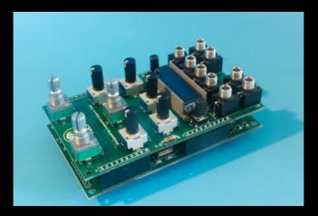
Place the front panel and carefully tighten the nuts for all potentiometers and jacks.
