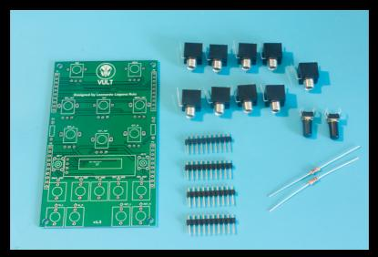
All components have to be mounted on the up-side (logo side) of the board.
