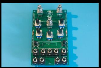
Once all of them are in place, put the front panel. Gently tight at least one nut of the jacks and one in the center potentiometer to keep it in place.
